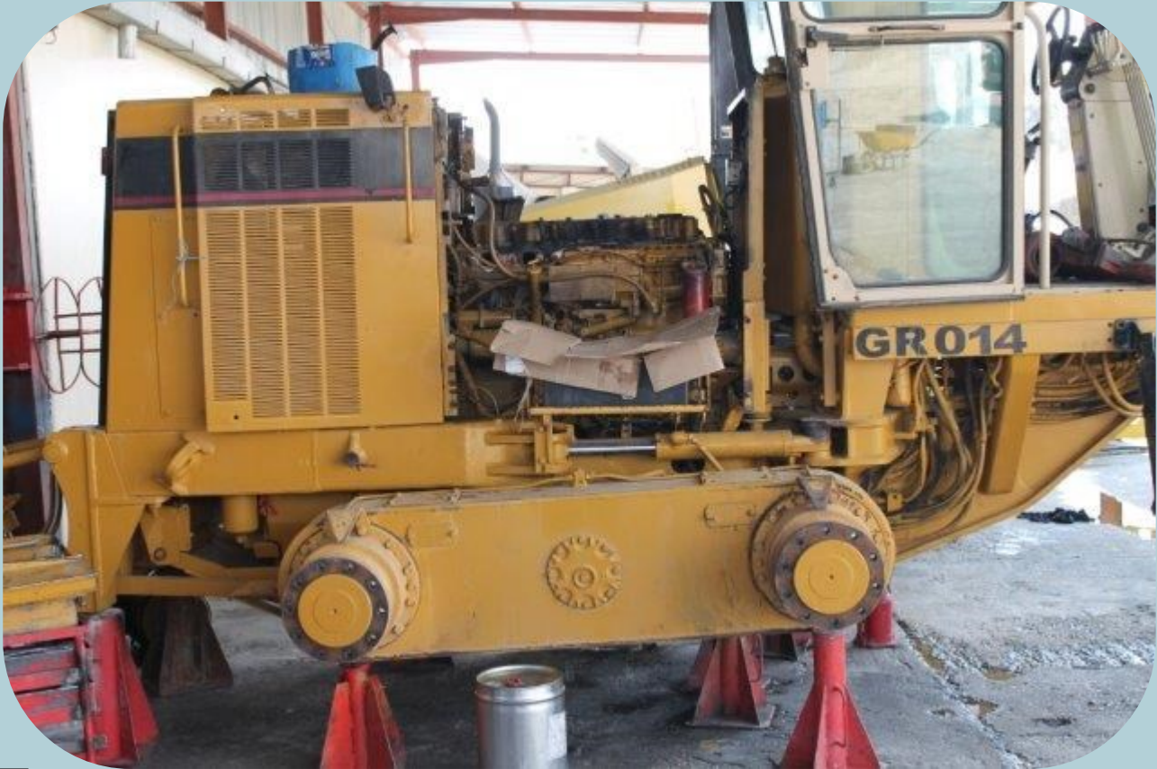
GRADER: Removed top and repairing oil leaks on Grader 14
